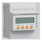
AIM-D100 type products are mainly used for monitoring of the positive and negative terminal-to-ground insulation resistance in the DC ungrounded systems. When the insulation resistance is lower than the set alarm value, an alarm message can be sent. The product is based on the unbalanced bridge principle.
